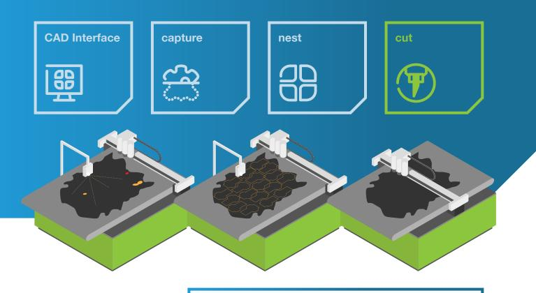
Leather pre-cutting modules combined with the cutting machine of your choice
